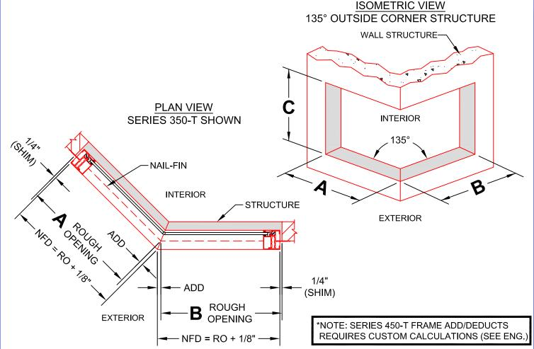
†IMPORTANT: 450-T SHIM SPACE VARIES PER WINDOW TYPE - (FIXED OUTSIDE GLAZED = .25"); (FIXED INSIDE GLAZED, P.O. w/BUTT HINGE, AND P.I. = .50"); (P.O. w/4-BAR HINGE = .625"). NOTE: 2X FOR DIM. REF. C
