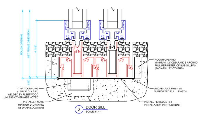
NOTES: 1. NET FRAME HEIGHT DOES NOT INCLUDE ARCHE-DUCT (.090 MATERIAL).
