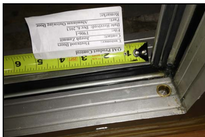
Fig. 15 – Sill weatherstripping and brass shootbolt cup
