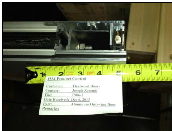
Fig. 8 – Stile and rail connection with multipoint shootbolt engaged.
