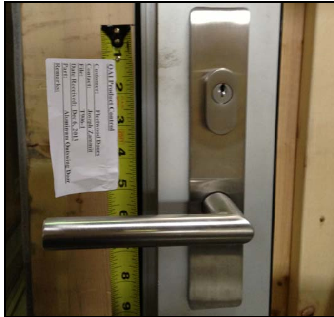
Fig. 13 – Multipoint lock and handle
