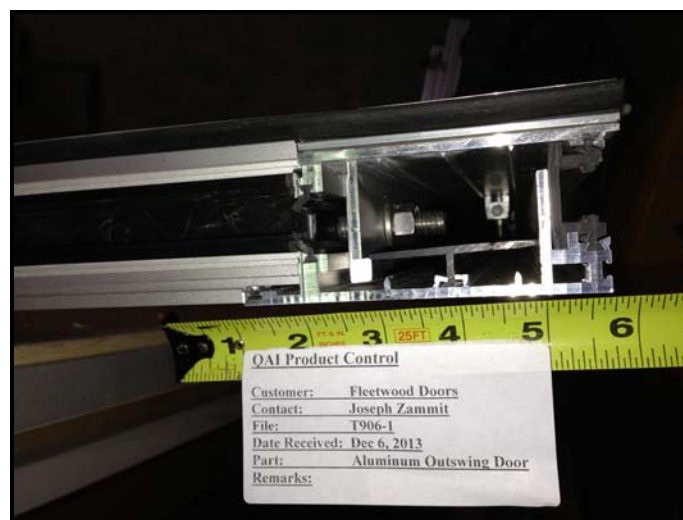
Fig. 6 – Stile and rail connection and frame profile
