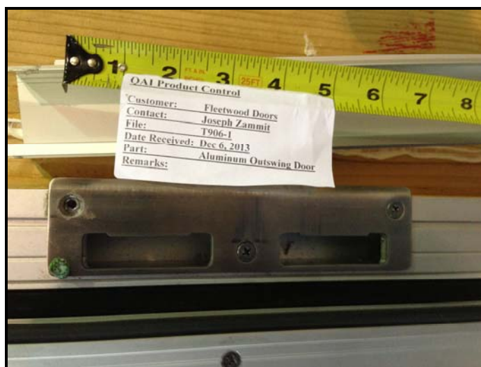
Fig. 18 – Latch and lock catch
