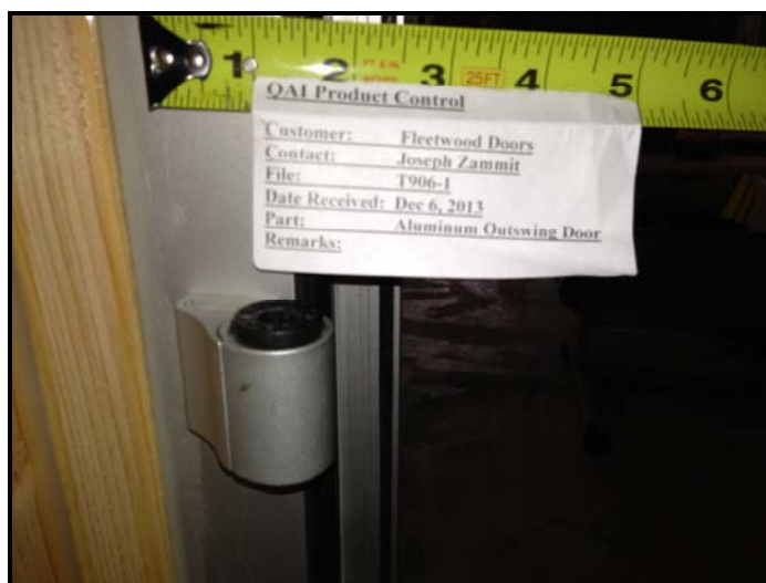
Fig. 21 – Frame hinge half
