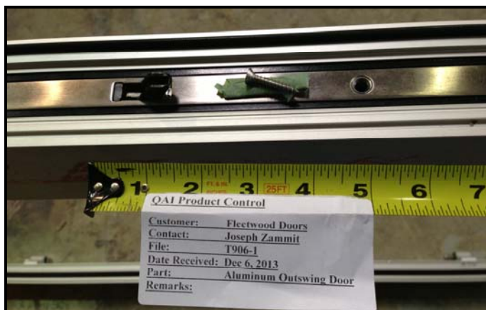
Fig. 12 – Tongue latch engaged position
