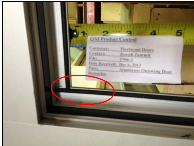
Fig. 4 – Slab frame glazing seal
