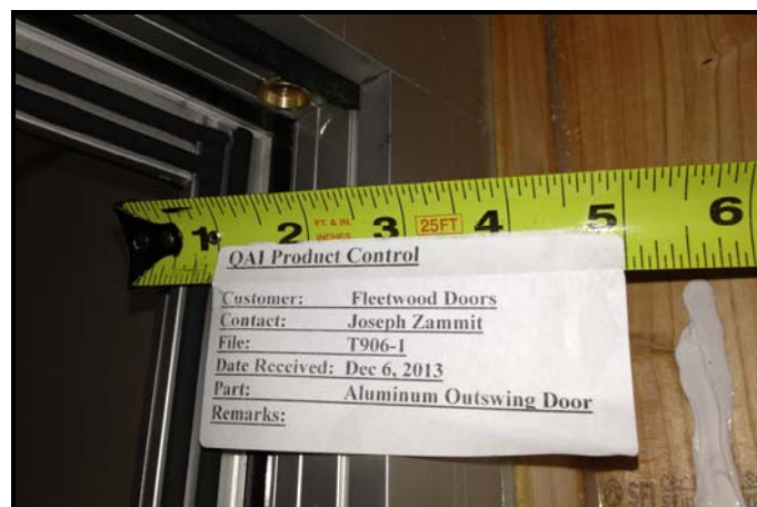
Fig. 14 – Frame weatherseals and brass shootbolt cup
