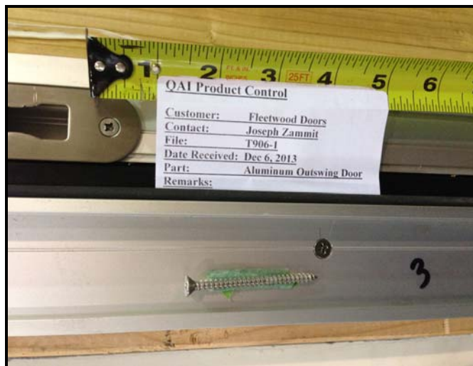
Fig. 1 – Installation screws through frame
