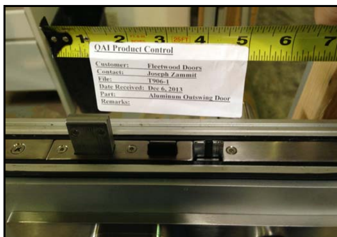
Fig. 11 – Multipoint latch with lock engaged
