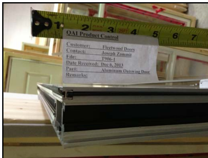
Fig. 7 – Slab weather seals (head to stile)
