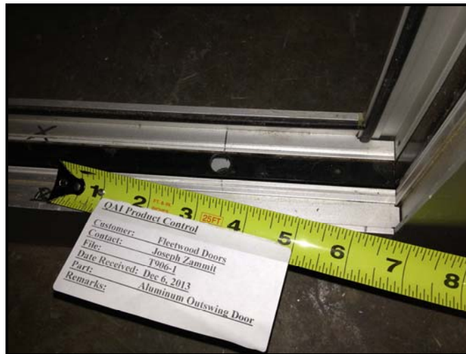
Fig. 5 – Slab drainage hole through thermal break
