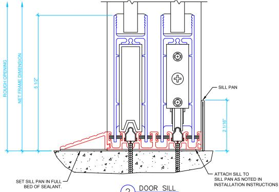
SILL DISCLAIMER: IT IS THE MANUFACTURERS DESIRE FOR THE INSTALLER TO NOT PIERCE THE SILL. IN SOME CASES THE CODE OF SPECIFICATIONS REQUIRE SUCH. IN THESE CASES THE INSTALLER IS RESPONSIBLE TO SEAL THESE BREACHES.
