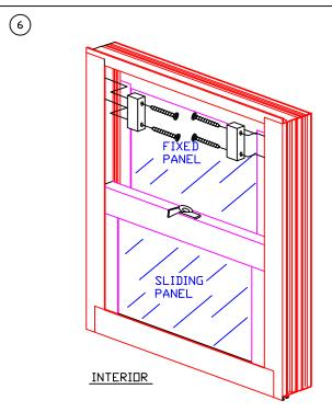
SECURE THE PANEL STOPS AS FAR AS POSSIBLE IN THE INTERIOR CHANNEL OF EACH JAMB WITH (4) #8 X 1-1/2" FLAT HEAD SCREWS.
