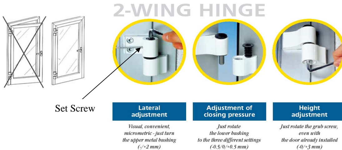
Figure 15: Hinge Adjustment
