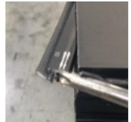
Figure 2: Remove retention clip
