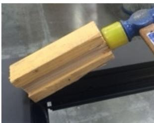
Figure 5: Use block of wood and mallet to separate stile from rail
