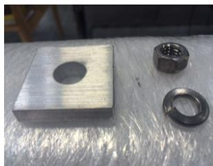
Figure 6: Back-up plate, lock washer & nut.
