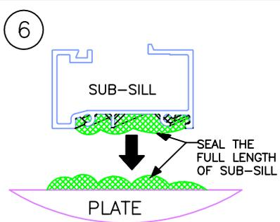
● SET THE SUB-SILL ON THE PLATE INTO A FULL BED OF SEALANT, AS SHOWN.
