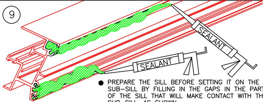
● PREPARE THE SILL BEFORE SETTING IT ON THE SUB-SILL BY FILLING IN THE GAPS IN THE PART OF THE SILL THAT WILL MAKE CONTACT WITH THE SUB-SILL, AS SHOWN.
