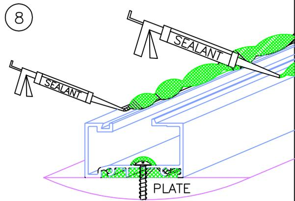
● PREPARE THE SUB-SILL PRIOR TO SETTING AND ATTACHING THE SILL BY RUNNING A FULL BEAD OF SEALANT ACROSS THE TOP OF THE SILL ON BOTH SIDES, FOR THE FULL LENGTH OF THE SUB-SILL.
