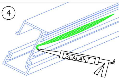
NOTE: BEFORE SETTING AND SECURING THE SUB-SILL INTO THE OPENING, COMPLETELY FILL THE CONTOURS IN THE BOTTOM OF THE SUB-SILL WITH COMPATIBLE SEALANT, AS SHOWN.
