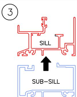
3. TAKE THE SILL AND ASSEMBLE THE FRAME, AS INSTRUCTED IN THE FRAME ASSEMBLY INSTRUCTIONS.
