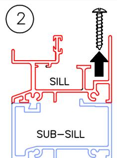
2. SEPARATE THE SILL FROM THE SUB-SILL, BY REMOVING THE SCREWS, AS SHOWN.
