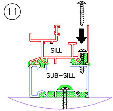
● RE-SECURE THE SILL TO THE SUB-SILL, USING THE SCREWS THAT WERE REMOVED IN THE BEGINNING, AS SHOWN.
