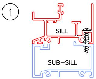
1. WHEN YOU RECEIVE YOUR K.D. WINDOW, THE SILL AND SUB-SILL WILL BE ATTACHED WITH SCREWS, AS SHOWN.
