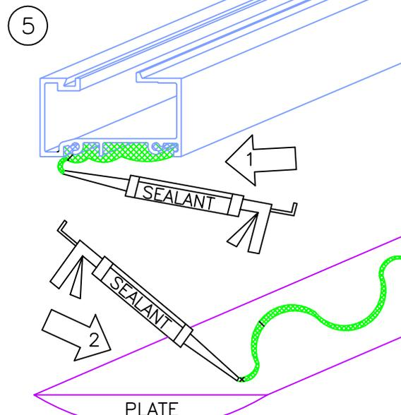
1. FILL IN THE BOTTOM OF THE SUB-SILL COMPLETELY WITH COMPATIBLE SEALANT, AS SHOWN.
