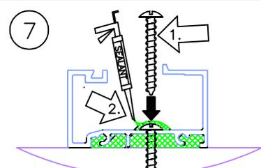
1. SECURE THE SUB-SILL TO THE PLATE WITH #8 X 2" TRUSS HEAD S.M.S. AT A MAX. OF 18" ON CENTER, AS SHOWN.
