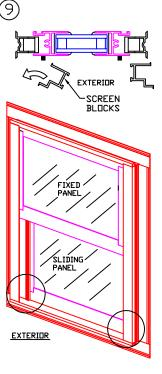
• INSERT A SET OF TWO SCREEN CENTERING BLOCKS INTO THE EXTERIOR CHANNEL OF EACH JAMB, ONE AT BOTTOM CORNERS ONLY.
