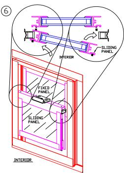
• INSERT DNE SIDE OF THE SLIDING PANEL INTO THE JAMB 2' OR 3' ABOVE THE TAKE-OUT CLIP. SWING THE OTHER SIDE INTO ALIGNMENT WITHIN BOTH JAMBS.
